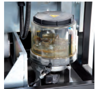
Automatic lubrication system for maintenance free operation
