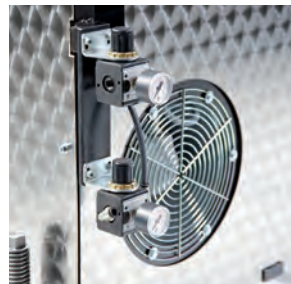
Pressure fan for cooling of machine
