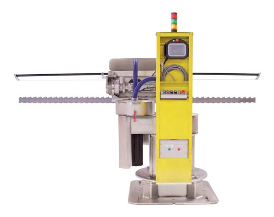
executed by the combination of the three, forward sideways and compensation movements. All three movements are executed by separate servo drives.
