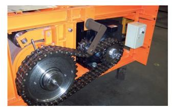
belt tensioning zone with its weight roller(s) distributing an even load onto the lehr belt, to compensate thermal stretch. The lehr belt drive is equipped with the main drive gear/motor assembly and a single chain providing the torque to the rubberized drive roller. Easy belt tracking adjustment is performed with the drive unit itself.
