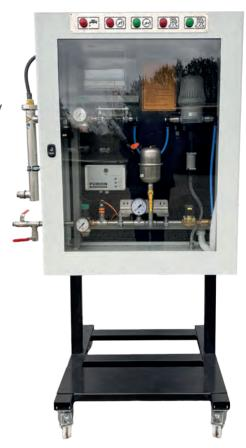
Thereafter, it sucks the coating material through the dosing unit, which again regulates the mixing ration. The storage / pressure tank will contain the mixture and by use of another pressure regulating valve, a constant flow and pressure of mixture is provided to the spray nozzle(s) itself. The failsafe and simplified unit fulfills today's requirements in container glass manufacturing.
