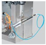
IR-temperature sensor Monitoring and possible control link to lehr (Pennekamp)
