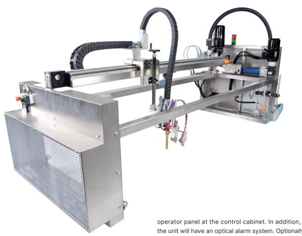
operator panel at the control cabinet. In addition, the unit will have an optical alarm system. Optionally, the cold end spray unit may be equipped with a pyrometer, in order to monitor the actual glass temperatures. In case of a deviation from the set temperature, it may generate an alarm or interfere actively in the prior glass cooling, such as lehr and/or blast cooling.
