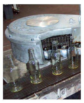
The ware transfer head is designed to be operated at a speed of up to 650 bottles per minute according to the bottle diameter. The transfer head is available with different numbers of fingers and designs.
